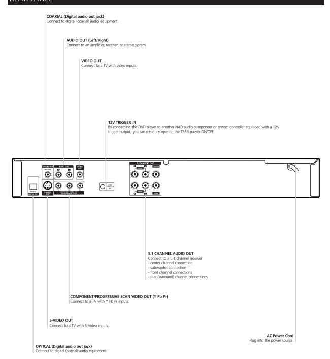
DO NOT TOUCH THE INNER PINS OF THE CONNECTORS ON THE REAR PANEL. ELECTROSTATIC DISCHARGE MAY CAUSE PERMANENT DAMAGE TO THE UNIT.
